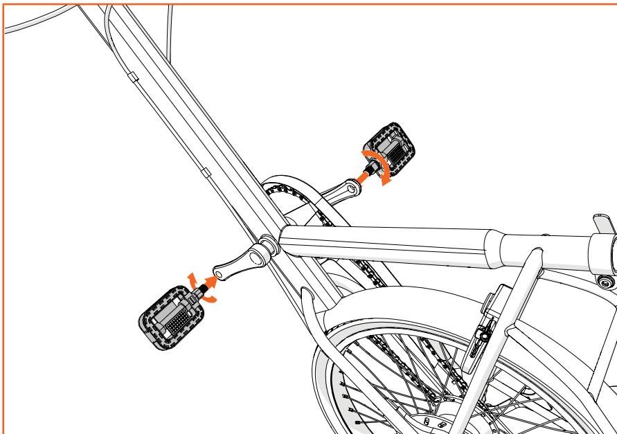
The left pedal is marked with an “L”. Hand-tighten it clockwise in the left-hand crank. Tighten the right pedal anticlockwise in the right-hand crank. Use wrench 15 to secure the pedals.
