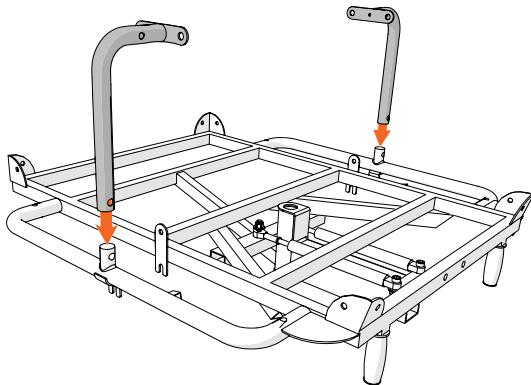
Place the side bars over the raised tubes on the top of the frame. Ensure that the screw holes in the bars and the tube are aligned. (It is possible that the bar may not exactly fit over the tube. In that case, sand down some of the paint to make it fit.)
