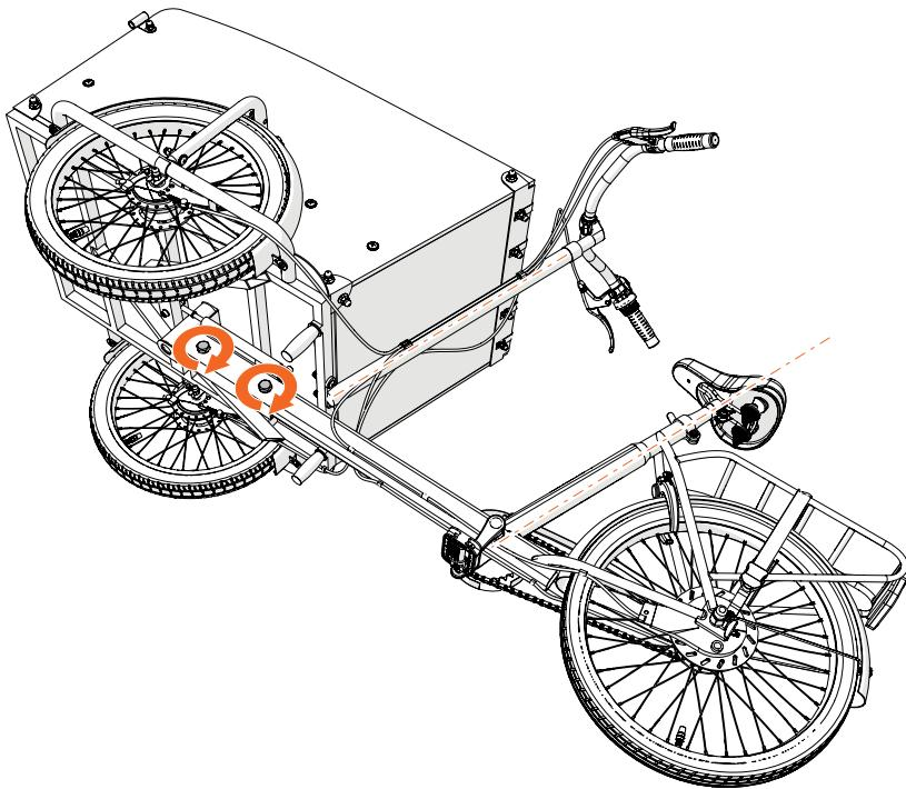
You might need someone to assist you with this step. Make sure that the seat post tube is aligned with the handlebar stem. Tighten the nuts as much as possible, while you (or possibly someone else) keep the frame aligned. Tighten the nuts again after having ridden the bike a few times.
