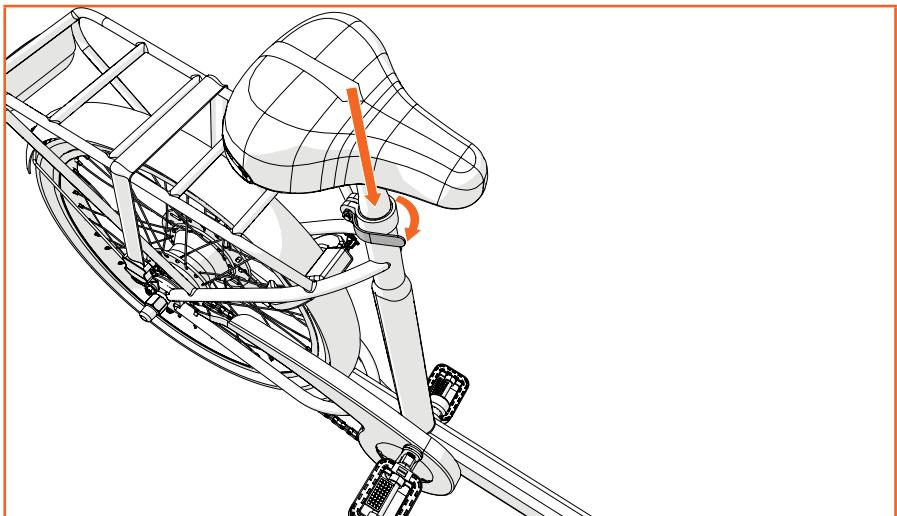
Slide the seat post in the seat tube and secure it with the quick release lever. Check whether the saddle is secured to the seat post and if necessary tighten the nuts some more.
