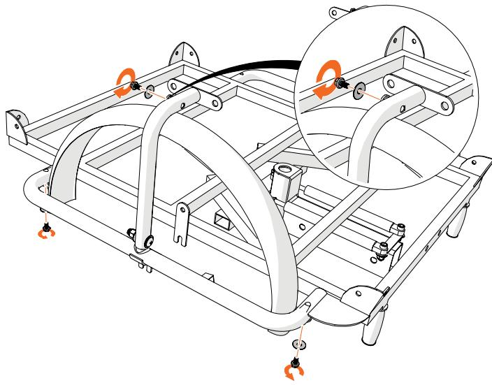
Unscrew the screw at the top of the bar. Then unscrew the screws in the frame. Position the fender and hand-tighten the screws. Alignment of the fenders will follow at a later stage.
