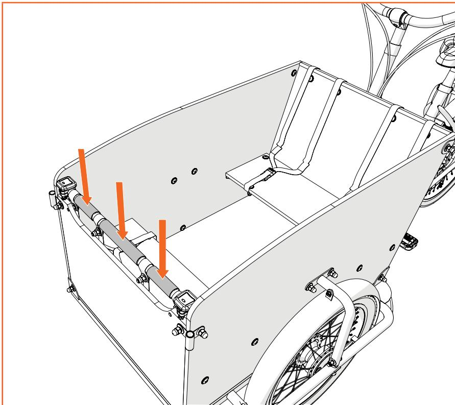
Place the foam sleeves between the seat belts around the front rod. This will prevent the seat belts from sliding during use.
