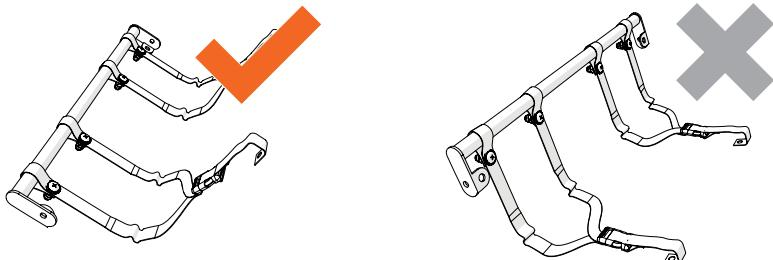
Attach two seat belts to the front rod using bolts kit G. Make sure that the nuts are positioned at the top.
