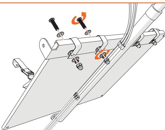
Install the rear panel simultaneously with two seat belts on the T-fitting. If a baby seat or toddler seat will be installed in the box, then there is no need to install the seat belt in that spot.
