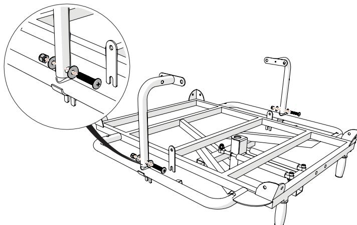
Use the nuts and bolts from kit F to secure the bars. Do not fasten them too tightly, this will follow at a later stage.
