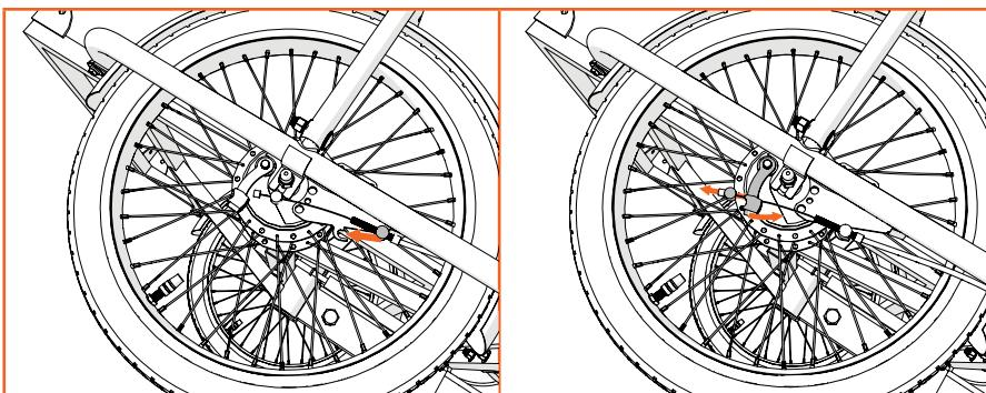
Ensure that the cables are properly routed through the holders on the T-bar. Please note: the cable marked with an "L" is longer. Guide this cable on the inside, along the anti-tip system to the eyelet (U-profile) and place the adjustment bolt in the slot of the brake arm. Squeeze the brake lever and hook the cable stopper behind it. Follow the same steps for the cable on the right. Secure the cables to the frame using the tie wraps included.
