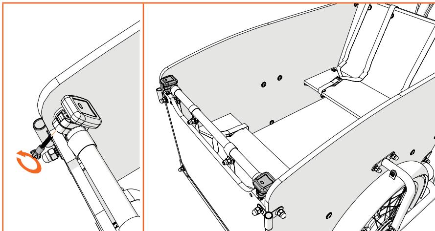
Pull the strip from the lights. Slide the light from the clamp, unscrew the clamp and place it on the front rod near the side panel. Tightly screw the clamp and position the light. Follow the same instructions for the light on the other side.
