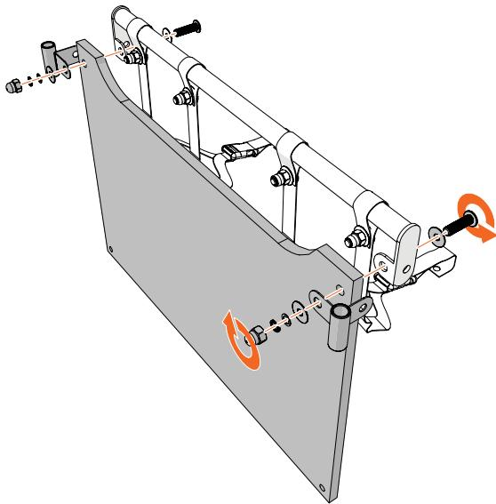
Attach the front panel to the front rod using bolts kit C. Make sure that the nuts are positioned on the outside of the box.
