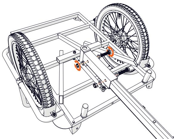
Use bolts kit H. Place the washer on the bolt. Then push the bolt through the frame. Place the second washer on the bolt. Place the nut and hand-tighten it. Do not fully tighten the nut just yet, this step will follow later. Use two 17mm ring spanners or wrenches.
