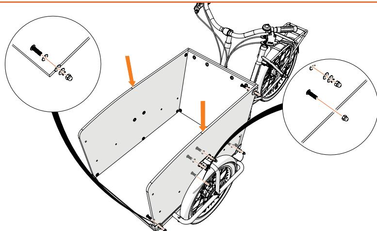
Lay the bottom panel in the front frame. Place the side panels and attach them to the front frame with bolts kit C. Use bolts kit D for the eyelet behind the wheel. Make sure that all nuts are positioned on the outside of the box.
