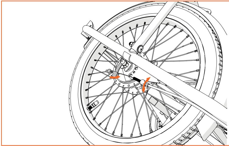
Afterwards, the brakes can be tightened or loosened with the adjustment bolt. Squeeze the brake lever and unhook the cable stoppers. Turn the adjustment bolt towards the rear frame to tighten the brake. Turn the adjustment bolt towards the front to loosen the brake. Squeeze the brake lever again and hook the cable stopper back in place. Take a look at the instruction video on our website as well.
