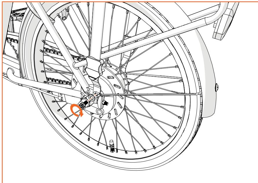
Loosen the screw and position the fender stay. Tighten the fender stay and follow the same instructions for the fender on the other side of the wheel.
