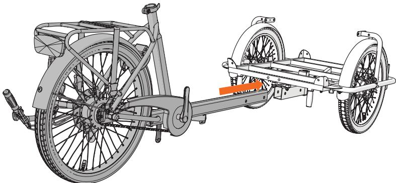
You might need someone to assist you with this step. Position the front frame upright and keep it horizontal. Slide the rear frame tube into the front frame. Check to ensure the tube is fitting tightly. If there is some play between the front and rear frame, use one of the two metal plates (included) to compensate for the play.
