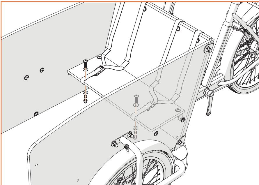
Secure the corner pieces to one of the benches using bolts kit C. Place the bench against the rear panel and use bolts kit B to attach the bench to the side panels. Ensure that the nuts are on the inside of the box. Attach the seat belts underneath the bench using bolts kit C. Make sure that the nuts are underneath the bench.
