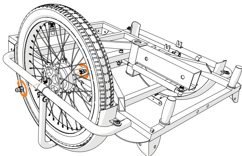
Turn the front frame upside down. Unscrew the bolts of the front wheel and place the axle in the frame and the brake bar in the bracket. Firmly tighten the bolts. Follow the same instruction for the other wheel.
