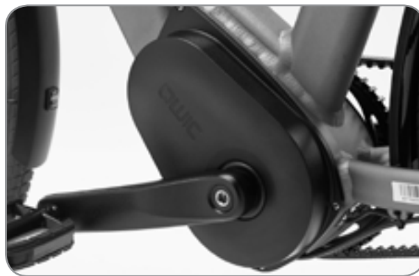
The Premium MN330 and MN380 are equipped with a Brose motor
