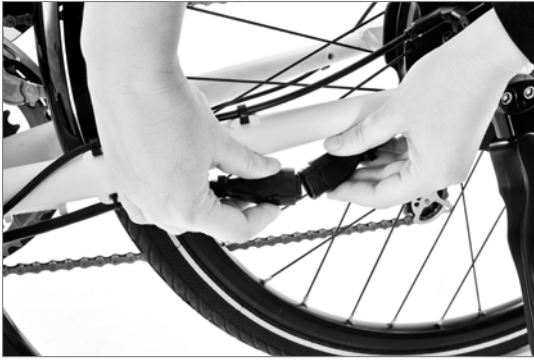
Disconnecting the cable
