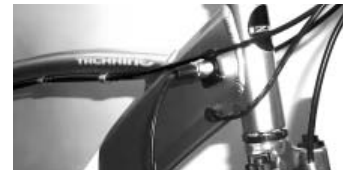
Electric Bikes with internal battery packs - Rotate the charger port cover and attach charger.
