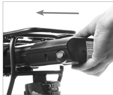
Reinstalling the battery
