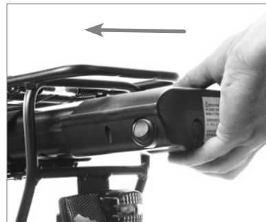
Reinstalling the battery
